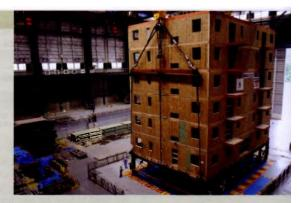
The team fully accepts that it could suffer significant damage and could even collapse completely. It is, after all, a destructive test. However, even a total collapse would provide useful data. [F]
